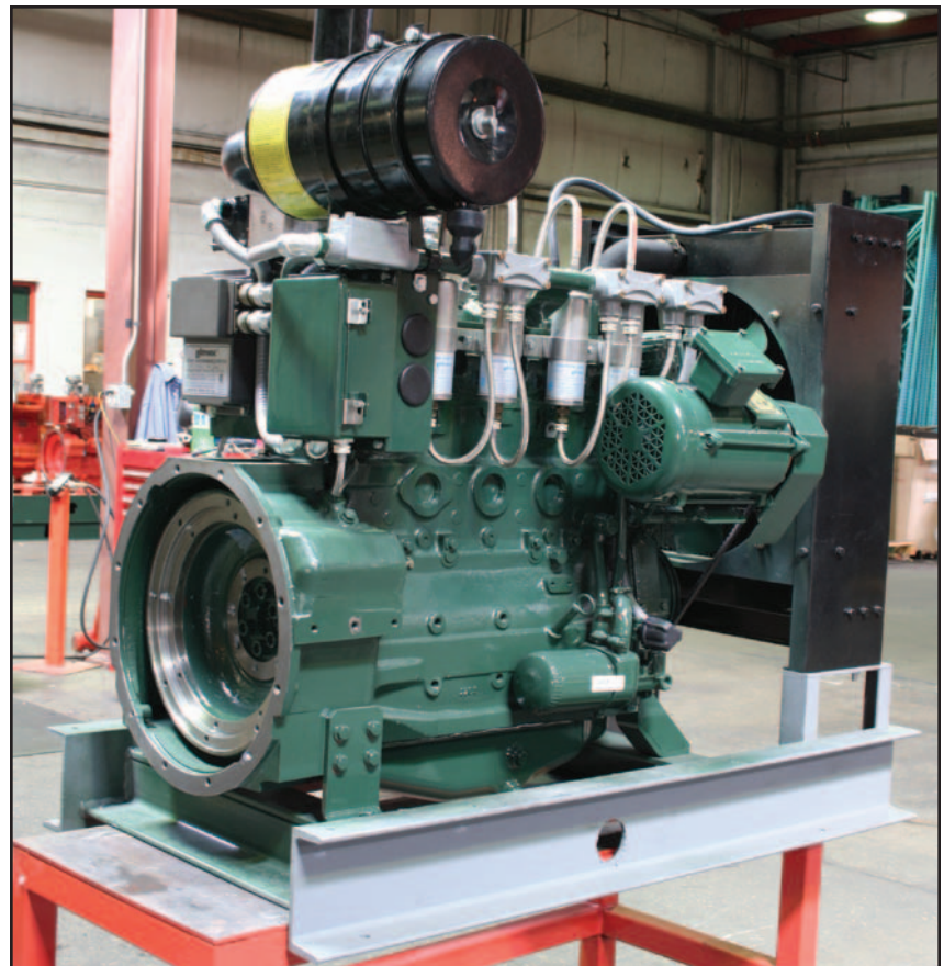
■ A VR260 power unit in final stages of assembly, this one with shielded ignition for Canada.
